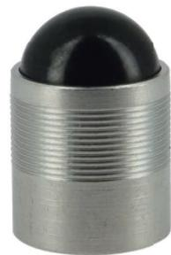
The insertion of the plug has to be made in a counterbored hole. The ball is pressed into the sleeve so that the top of the ball is slightly below the top of the sleeve, and allows expansion of the sleeve.
